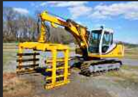
Plasser Australia Tie Handling Machine
